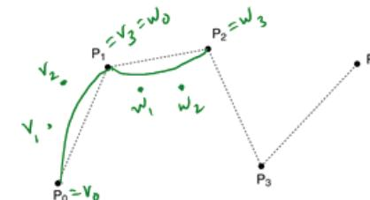
We call this curve a **spline**. The endpoints of the Bézier segments are called **joints**.
