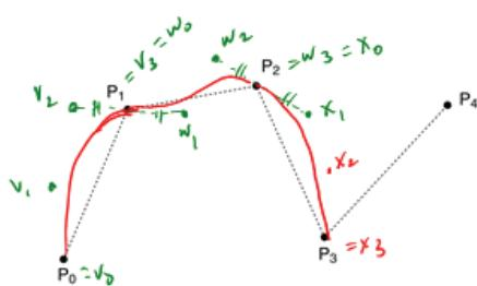
We can specify the Bezier control points directly, or we can devise a scheme for placing them automatically...
