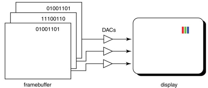
A display that allows 256 voltage settings for each of R, G, and B is known as a **full-color system**.
