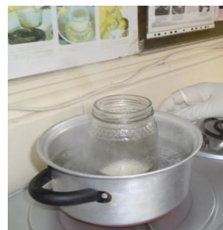
Figure 2: Low cost, low-tech flash heat pasteurization being used at a human milk bank. A milk jar without a lid is placed in a pan of water, which is then heated. When water reaches a rolling boil, milk reaches a temperature high enough to deactivate contaminants like HIV and other pathogens.
