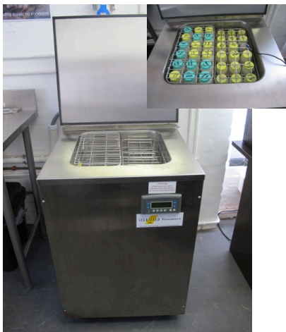
Figure 1: A high-end commercial pasteurizer. It provides temperature monitoring and archival on a computer, via a temperature probe that is connected to the computer. Milk bottles placed in the pasteurizer are shown in the inset.
