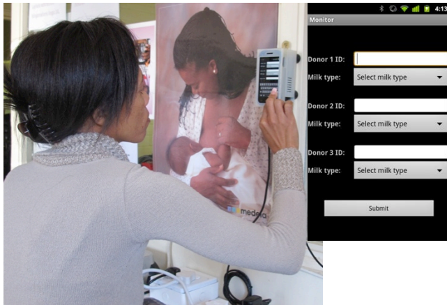
Figure 10: The system deployed at the Neonate ICU of King Edward Hospital. The Milk bank technician is entering donor information on the mobile app. Up to 3 donors can be entered on this screen (inset is a screenshot). Donor information includes a unique donor ID and a milk-type, which could be term or pre-term milk. This corresponds with the donor mother having delivered a term or a pre-term baby.
