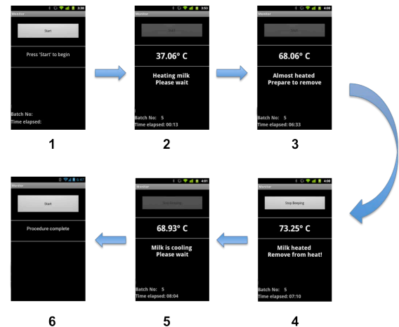
Figure 4: Screenshots of the Android application that guide the user through the pasteurization process. 1) User places water and milk jars in the water bath and turns the stove on. Clicking the “Start” button on the app starts the pasteurization monitoring process. 2) A unique batch ID is generated for the procedure. Rising temperature is displayed on the screen along with the time elapsed. 3) Phone beeps twice to alert user 5° before high temperature threshold of 73° C is reached, visual indicator changes accordingly. 4) Visual indicator changes at 73° C and phone starts to beep continuously until user removes jars from water bath. 5) Beeping stops and visual indicator changes to indicate cooling when app detects drop in temperature. 6) Procedure is complete when temperature drops to 25° C.
