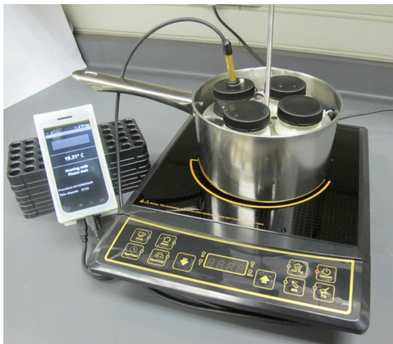
Figure 6: The mobile milk pasteurization equipment. A stand holds 4 glass jars. The temperature probe connected to the mobile phone, is secured on the jar containing water; the other jars contain milk. The stand with jars containing liquid is placed in a water bath that gets heated on an induction stove. The white enclosure on the left side of the picture hosts the mobile phone and the USB Bridge that connects the probe to the phone.
