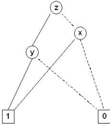
d) With 6 edges, the reduced OBDD with orderings [z,x,y] and [z,y,x] have the minimal number of edges.
