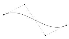
We'd like to have a spline that is **interpolating**, that is, that always passes through every control point.
