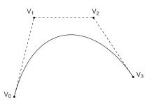
In general, the *n*th derivative at an endpoint depends only on the n+1 points nearest that endpoint.
