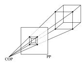
The center of projection is exactly the same as the pinhole in a pinhole camera.
