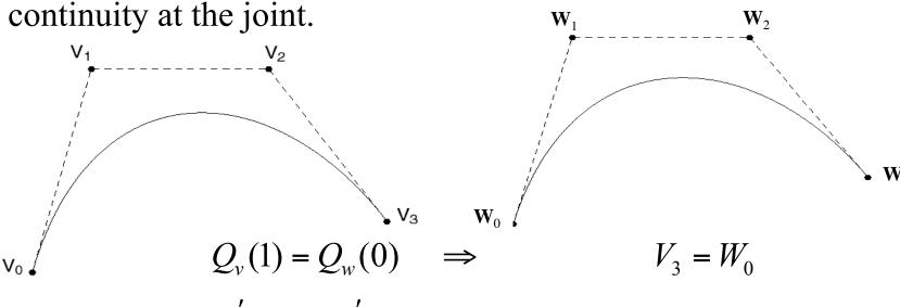
$$Q'(0) = 3(V_1 - V_0) \qquad Q'(1) = Q''(1) \Rightarrow V_3 - V_2 = W_1 - W_0$$
