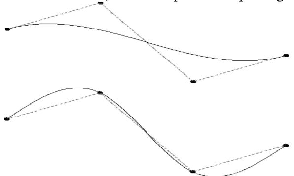
We'd like to have a spline that is **interpolating**, that is, that always passes through every control point.
