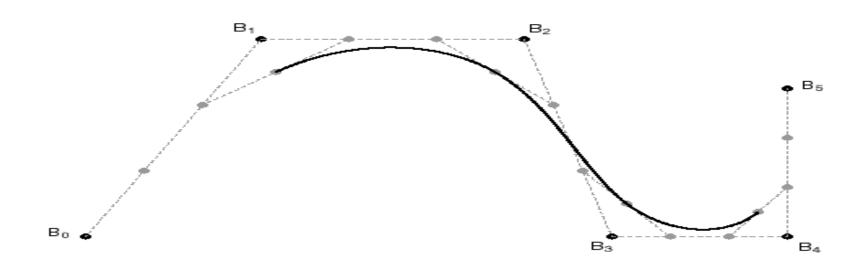
These are called **B-splines**. The starting set of points are called **de Boor points**.
