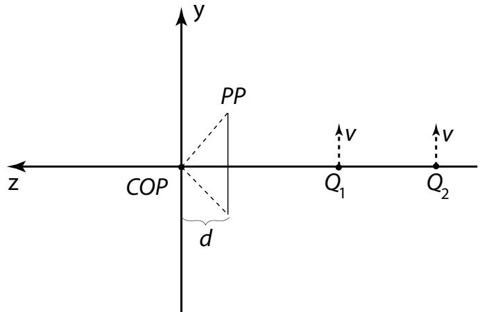
Compute the projections  $q_1$  and  $q_2$  of points  $Q_1$  and  $Q_2$ , respectively. Then, compute the velocities,  $dq_1/dt$  and  $dq_2/dt$ , of each projected point in the image plane. Which appears to move faster? Show your work.
