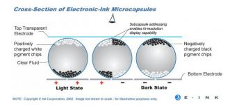
This kind of display is **bistable**, which means that the image holds after removing the voltage.
