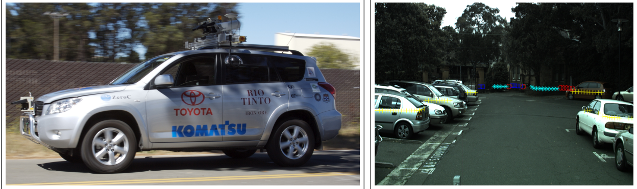
Figure 4: (left) One of the vehicles we will use to collect data for semantic mapping in urban environment. The vehicle, built by the Australian Centre for Field Robotics, is equipped with multiple cameras and laser range-finders. (right) Camera image along with a projected laser scan. Colors of mapped laser returns indicate the type of object each return points at (see also [32]).
