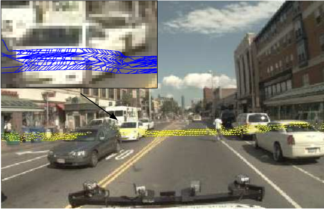
Fig. 6. An example of image from the Boston dataset displayed with the associated projected laser returns (in yellow). A part of the CRF network built from these laser returns is displayed in blue in the inset in the top left corner. The image in this inset corresponds to a magnification of the area indicated by the arrow.
