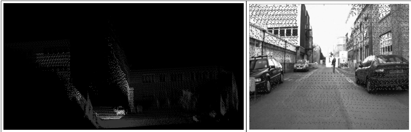
Fig. 6. Camera-laser cross-calibration: a typical 3D laser point-cloud (left). Laser points within the camera frustum are highlighted (white) and projected into the corresponding camera image (right).
