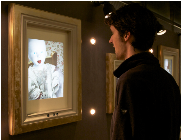
Figure 12: Mimicry, an application case study using our approach. An observer can simply step in front of the picture frame and the character depicted in the virtual painting will start mimicking the person’s facial expression in realtime. The sensor is embedded in the frame. See also accompanying video.
