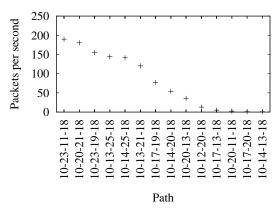
Figure 6: Measured capacity on various 3-hop paths from node 10 to node 18 (27-Jun-17:00). The units are packets per second; each packet contains 124 bytes of 802.11 payload.
