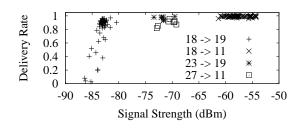
Figure 12: Delivery rates over 100 msecs versus average signal strength of received packets for four example links on the indoor network (6-Mar-18:30-50-byte). For clarity, only 1 in 50 of the data points are shown for each link. Signal strength more accurately reflects link distance than delivery rate.
