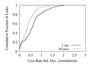
Figure 9: The indoor network's cumulative distribution of the standard deviation of short-term link *loss* rates. For each link, the loss rate is calculated over 1- and 10-second intervals, and the standard deviation is normalized by the link's mean loss rate (8-Feb-13:30-50-byte). Many links show significant variation in short-term loss rates over time.
