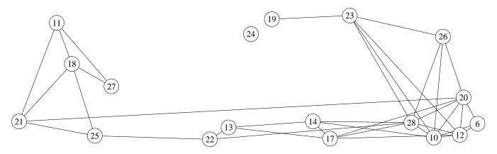
Figure 2: Indoor network links with greater than 90% delivery rate in both directions show that the network is well connected (8-Feb-13:30-50-byte). Node 24 was not functioning during this experiment. For clarity, node positions have been slightly changed from Figure 1.
