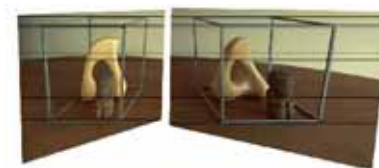
(c) Image pair transformed by the similarity H_L and H_R . Note that the image pair is now rectified (the epipolar lines are horizontally aligned).
