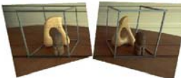
(d) Final image rectification after shearing transform H_1 and H_2 . Note that the image pair remains rectified, but the horizontal distortion is reduced.
