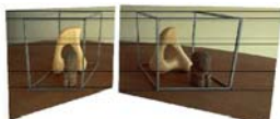
(c) Image pair transformed by the similarity H_1 and H_2 . Note that the image pair is now rectified (the epipolar lines are horizontally aligned).
