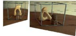
(b) Image pair transformed by the specialized projective mapping H_1 and H_2 . Note that the epipolar lines are now parallel to each other in each image.
