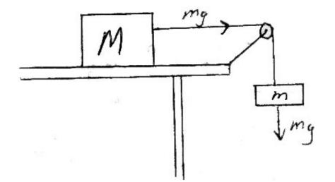
Friction, Air friction, Mass of pulley, Inelastic string, ...
