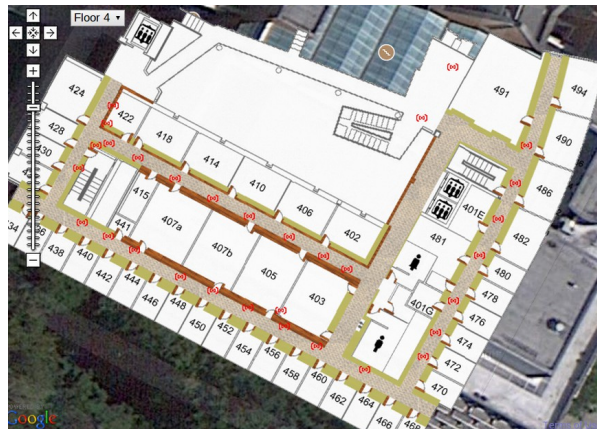
Fig. 1. RFID antenna deployment map on the 4th floor of the UW CSE building.
