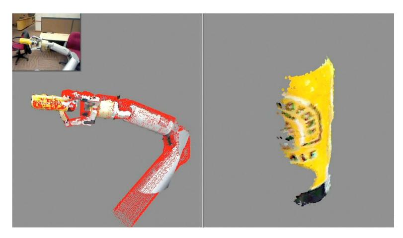
EKF with articulated ICP over manipulator joint angles, camera pose and pose of (partial) object
