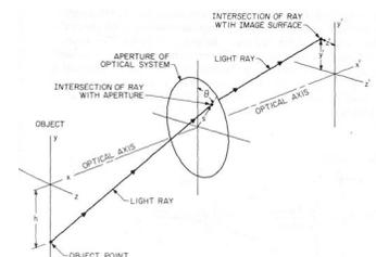
Figure 3.1 A ray from the point  $y = h$ ,  $x = 0$  in the object passes through the optical system aperture at a point defined by its polar coordinates,  $(s, \theta)$ , and intersects the image surface at  $y', z'$ .
