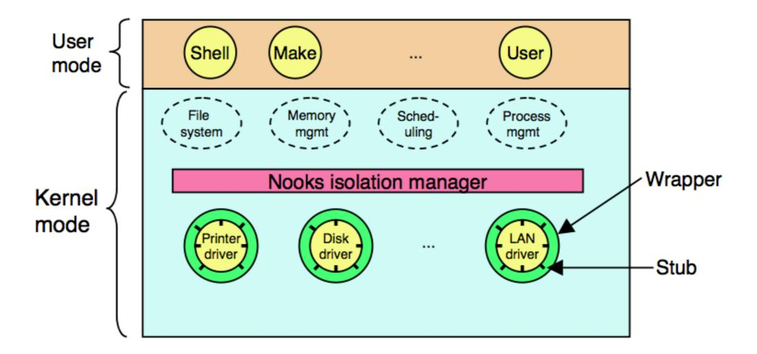
Each driver is wrapped in a layer of protective software that monitors all interactions between the driver and the kernel
