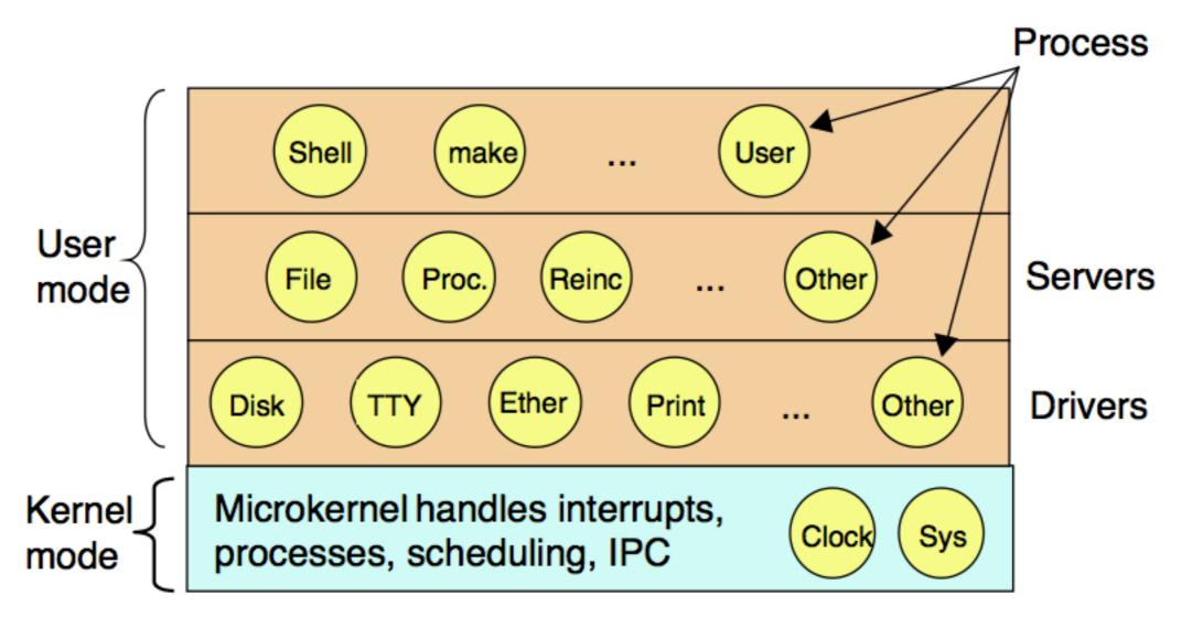
A tiny kernel runs in kernel mode with the rest of the OS running as a collection of fully-isolated user-mode server and driver processes
