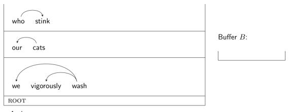
Actions: SHIFT SHIFT LEFT-ARC LEFT-ARC SHIFT SHIFT LEFT-ARC SHIFT SHIFT RIGHT-ARC
