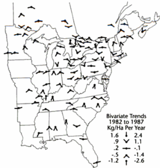
FIGURE 3.39. Bivariate map of NO 3 and SO 4 trends. The original Carr et al. version of this map used a wheel with eight spokes, rather than a simple dot, as the center of each glyph. When large enough, this added feature facilitates judgment of specific values. After Carr et al. (1992, Fig. 7a, p. 234). Adapted by permission of the American Congress on Surveying and Mapping.
