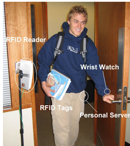
Figure 3. A user walking through a doorway with several tagged objects. An RFID reader is visible to the left (white box on black stand); tags are visible on the notebooks in his hand; his personal server is in his front left pants pocket; and, our wristwatch UI is on his left wrist (images of the personal server and wristwatch are in Figure 4).
