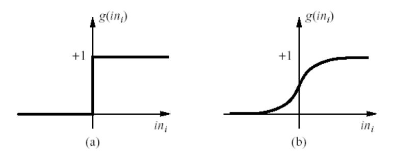
(a) is a step function or threshold function
