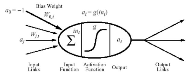
A gross oversimplification of real neurons, but its purpose is to develop understanding of what networks of simple units can do
