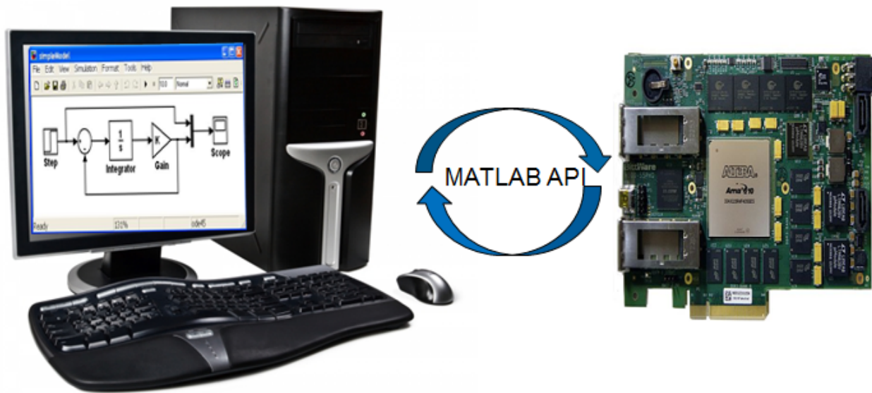
Figure 10-6: Hardware in the Loop Host-Target Setup
