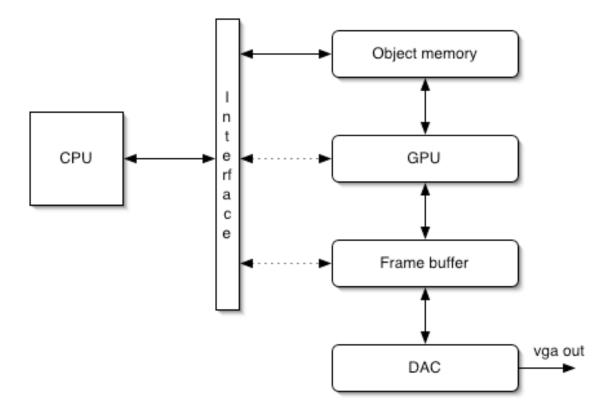
Graphics cards render a sequence of objects. These objects are passed to the graphics card over a FIFO link, usually in a DMA like fashion. They are stored to an object memory, essentially a polygon list. The CPU also controls the GPU and frame buffer, but this control is limited (reading and writing the frame buffer, and controlling the GPU).
