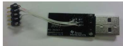
Header to JTAG signals has to be manually added
