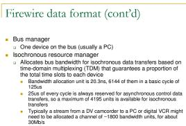
Asynchronous transfers can have multiple data packets per basic cycle, within the 25us reserved for this type of signalling
