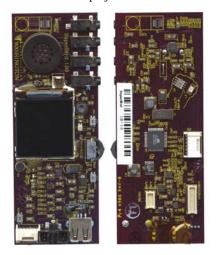
Figure 3. The top and bottom of the Intel iMote2 "SuperBird" board containing LCD, microphone, speaker, jog dial (near center), USB connector (left, on bottom right), and heart rate sensor (diagonally arranged area on right).
