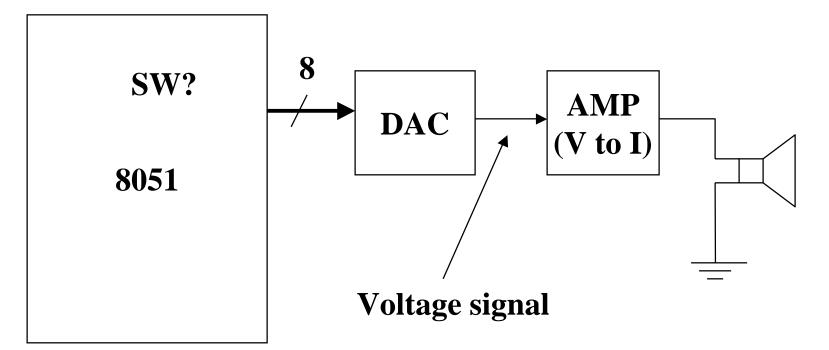
Speaker cares about current, not voltage What is algorithm to superimpose 1KHz tone with 500Hz tone With a sampling rate of 10KHz
