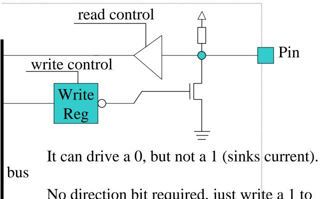
No direction bit required, just write a 1 to the port register to use as input pin.
