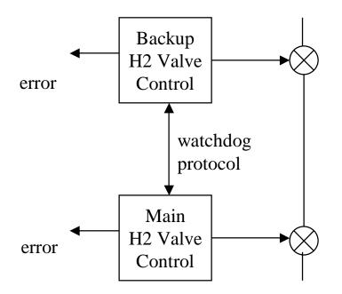
If the handshake fails, then either one or both can shut off the gas supply. Is this a single fault tolerant system?
