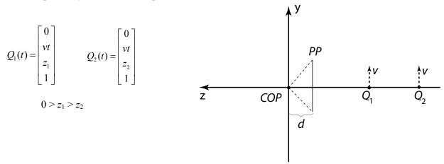
Compute the projections  $q_1$  and  $q_2$  of points  $Q_1$  and  $Q_2$ , respectively. Then, compute the velocities,  $dq_1/dt$  and  $dq_2/dt$ , of each projected point in the image plane. Which appears to move faster? Show your work.
