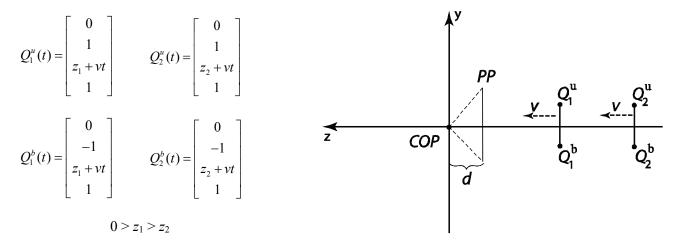
Compute the projected lengths,  $l_1$  and  $l_2$ , of the line segments. Then, compute the rates of change,  $dl_1/dt$  and  $dl_2/dt$ , of these projected lengths. Are they growing or shrinking? Which projected line segment is changing length faster? Show your work.
