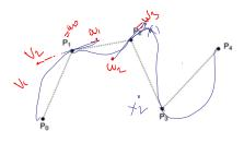
We can specify the Bezier control points directly, or we can devise a scheme for placing them automatically...
