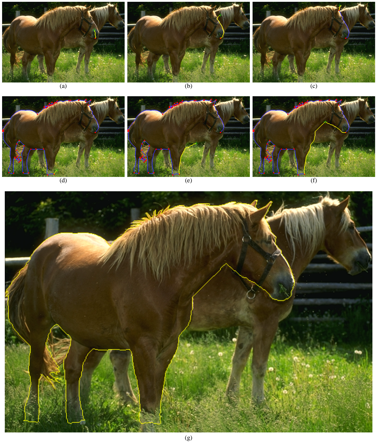
Figure 1: Selected frames from an example live-wire segmentation where both the object boundary extracted and the background are complex. The red dots are seed points, the green crosshair is the free point, the blue contour segments correspond to portions of the “set” boundary, and the yellow contour segment is the live-wire boundary segment. (a-c) Selected frames from the first couple of seconds of the interactive segmentation process. (d-f) Selected frames from the last couple of seconds of the process. (g) The final object boundary contains 2348 pixels. (Image size: 640×420)
