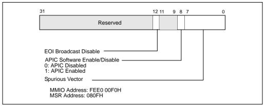
Figure 2-7. Spurious Interrupt Vector Register (SVR) of x2APIC
