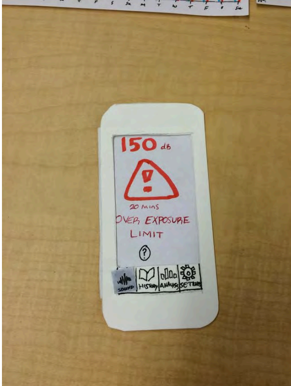
1.h – once the exposure level is reached, the screen changes to reflect the urgency of the conveyed information.
