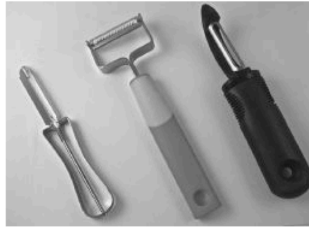
FIGURE 6.3. Three Vegetable Peelers. The traditional metal vegetable peeler is shown on the left: inexpensive, but uncomfortable. The OXO peeler that revolutionized the industry is shown on the right. The result of this revolution is shown in the middle, a peeler from the Swiss company Kuhn Rikon: colorful and comfortable.
