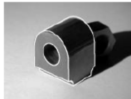
Figure 20: The pose computed from six point correspondence and one ellipse-circle correspondence using the generalized methodology.
