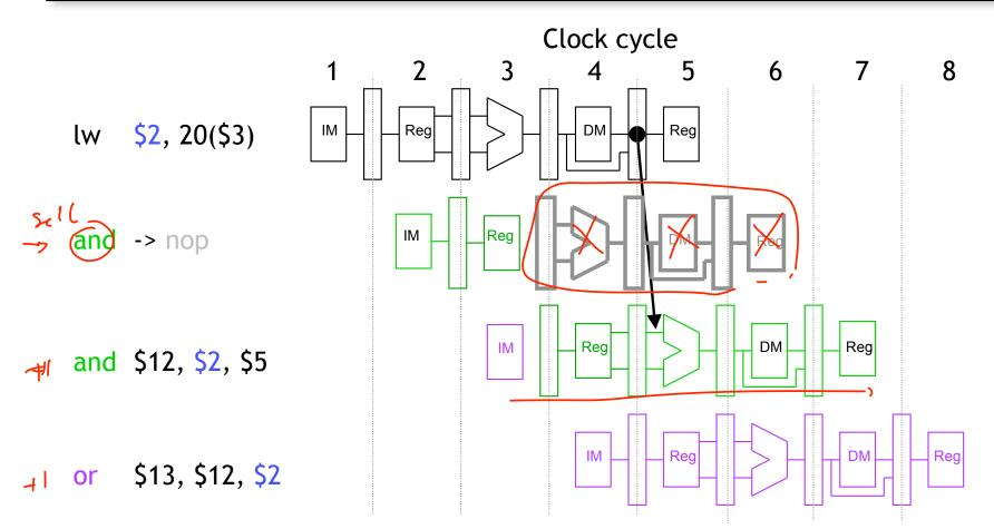
The effect of a load stall is to insert an empty or nop instruction into the pipeline then Bypass Rs from EX/MEM stage latch 3
