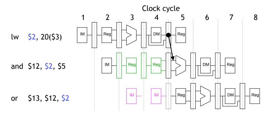
Those units aren't used in those cycles because of the stall, so we can set the EX, MEM and WB control signals to all 0s.
