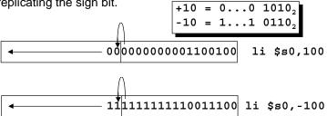
Sign extend is also applied when loading bytes and halfwords, i.e. lb and lh
