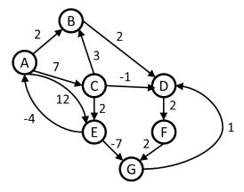
(a) Even though the graph has negative weight edges, step through Dijkstra's algorithm to calculate supposedly shortest paths from A to every other vertex. Show your steps in the table below. Cross out old values and write in new ones, from left to right within each cell, as the algorithm proceeds. Also list the vertices in the order which you marked them known.
