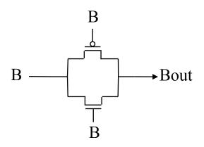
❖ Build an XOR gate from transistors. Assume you have two inputs, A and B, as well as their inverses (Ā and B).
