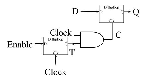
\* If gate delays are 1.0ns each,  $T_{\text{setup}}$  is 0.5, and  $T_{\text{hold}}$  is 1.5, what is the best clock period for this computation?
