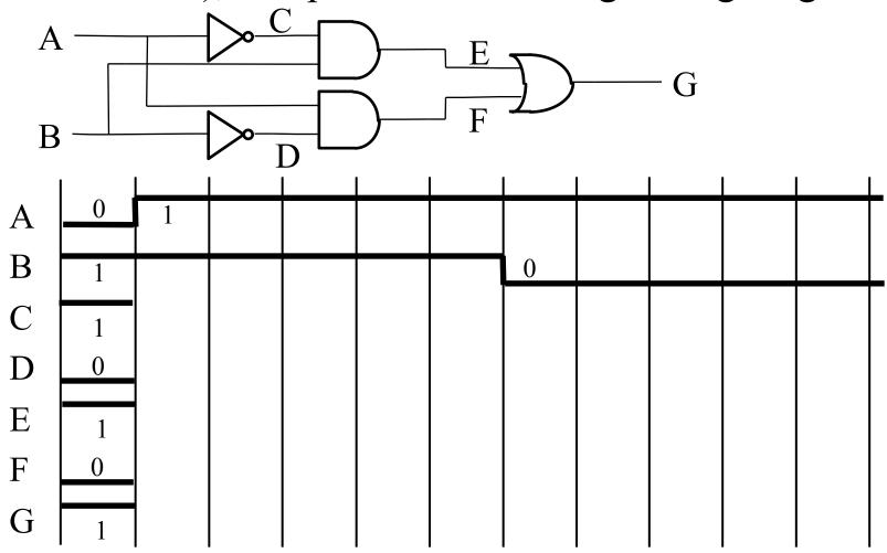
\* Write the Verilog for a 2-input gate that is TRUE when an odd number of inputs are true.
