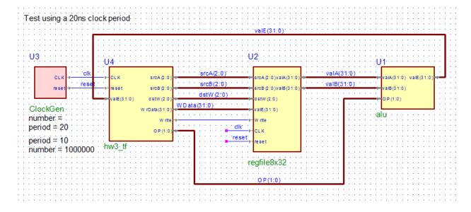
The test fixture executes "instructions" which tells the ALU what operation to perform and which registers to use for the inputs of the operation. It also tells the register file when and what to write (not the ALU result). Single-step your test fixture and write down what is executed by the test fixture.
