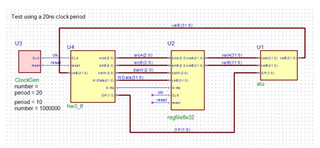
The test fixture executes "instructions" which tells the ALU what operation to perform and which registers to use for the inputs of the operation. It also tells the register file when and what to write (not the ALU result). Single-step your test fixture and write down what is executed by the test fixture.
