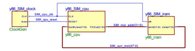
For the first version of the Y86 processor, you will only need to handle the following instructions: OPL (ADDL, SUBL, ANDL, XORL), RRMOVL, and IRMOVL, in addition to HALT and NOP. OPL instructions read values from the register file, use the ALU to perform an operation, and store the result back to the register file. The RRMOVL instruction simply moves a value from one register to another, and the IRMOVL moves data stored in the instruction itself to a register.
