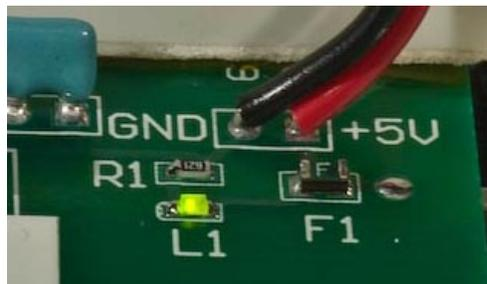
There is a fuse and an indicator light on your prototyping board. If you do accidentally wire up GND to VDD, you will mostly likely blow the fuse "F1" and the light "L1" will go off.
