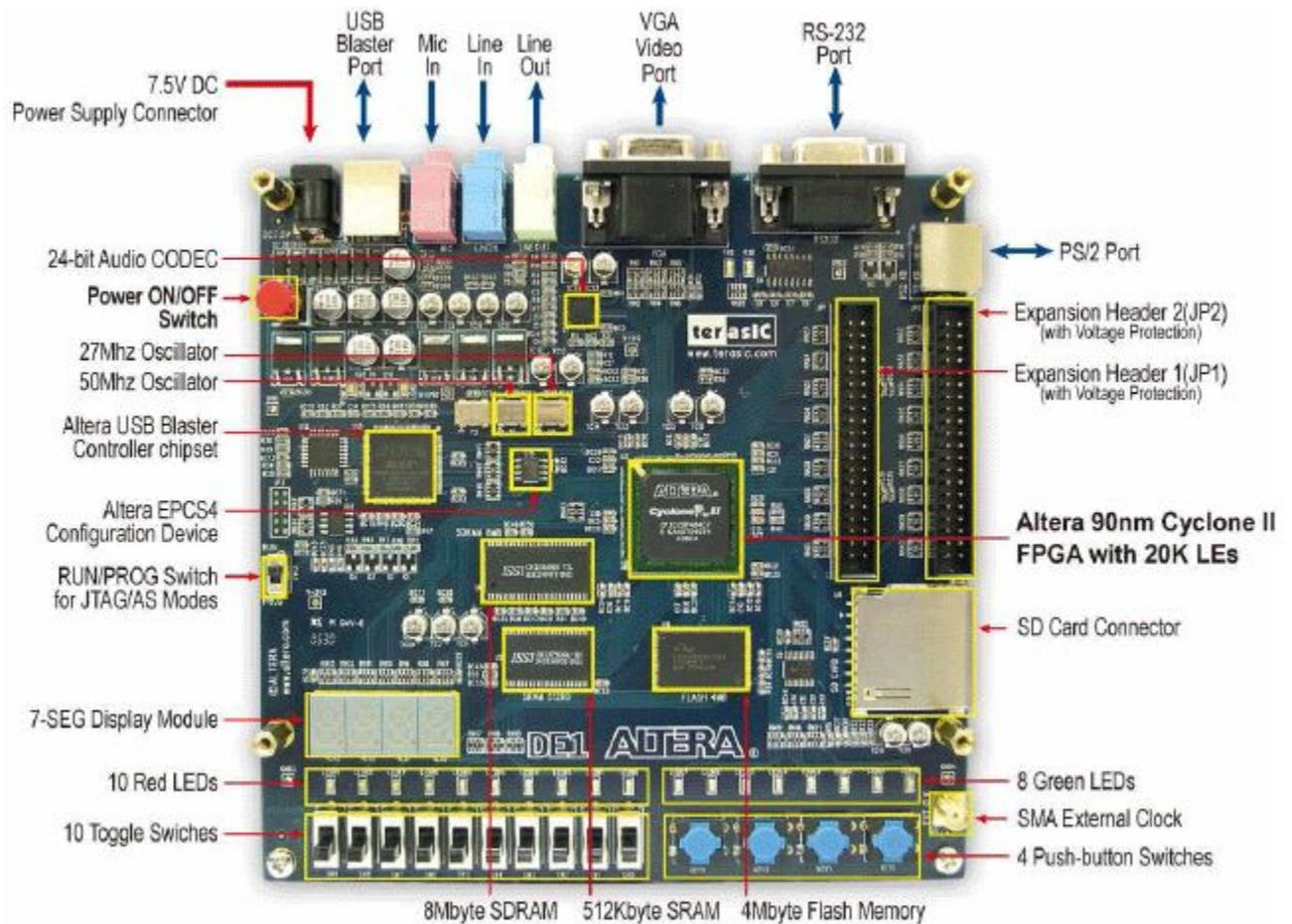
The picture above is a diagram of the prototyping board with most of the major components highlighted. For the first few labs you will be using the various input/output devices located directly on the board such as the switches and LEDs. Further details will be provided in each lab. Take note of the large FPGA (Field Programmable Gate Array) that is highlighted on the board. Later on in the quarter you will be programming this and directly interfacing with all the devices on the board.
