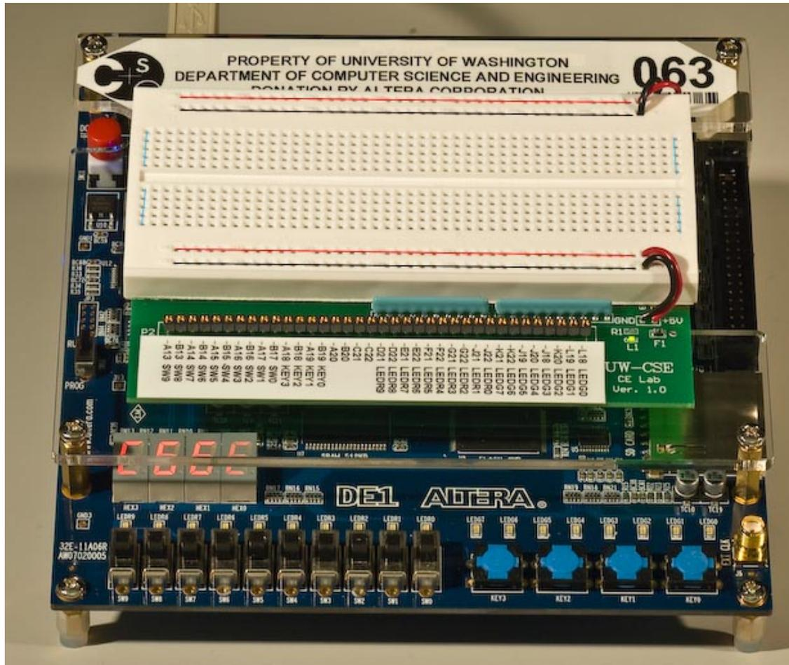
The red line marks where VDD runs across the board, and the black line marks where GND runs across the board. The holes on the board are interconnected as the blue line shows, up-and-down for each 5-hole segment.
