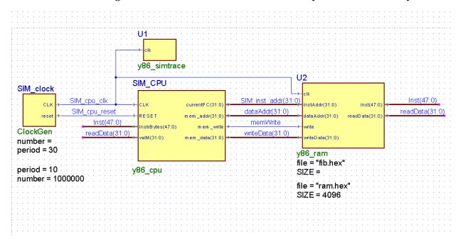
Let's start with the rmmovl instruction that writes data in the A register to the memory address formed by adding the B register to the constant in the instruction. First, you should use the ALU to perform this add instruction. You will note that the y86v1 CPU that we give you makes this convenient: setting the ALU input muxes appropriately allows the ALU to perform this. Then all you have to do is connect the appropriate signals to the memory ports.
