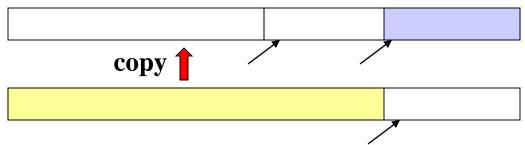
If right-side finishes first, copy dregs directly into right side, then copy auxiliary array
