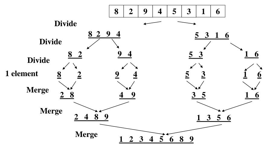
We need another array in which to do each merging step; merge results into there, then copy back to original array 35
