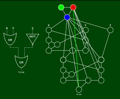
If we can find a solution to 3-COLOR, we can solve CIRCUITSAT quickly.
