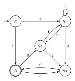
(b) [15 Points] The NFA below, which is nearly what we get by applying the construction described in class (the only simplification is using three states rather than four to represent the sub-expression 00) to the regular expression  $(\varepsilon \cup 0)(1 \cup 00)^*$ :
